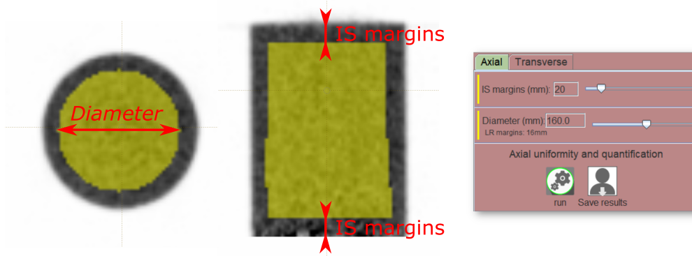
Figure 1.3: Definition of the ROIs for the calibration and axial uniformity test
