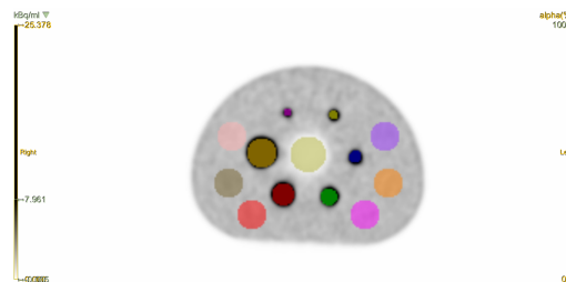
Figure 2.3: The thirteen VOIs drawn in the NEMA IEC NM/PET Body Phantom Set™.
